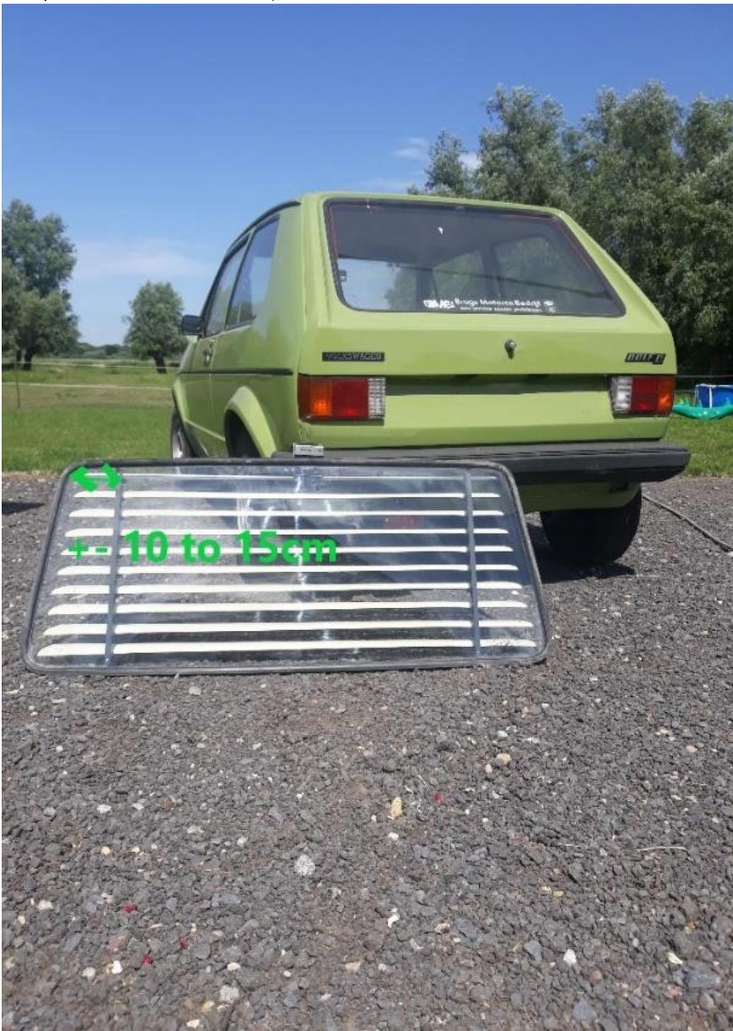
Make sure the width between the 2 brackets is the same above and below. This is very important. If the brackets don't have the same width above and below, the blind slats will have a ugly curve when installed.
